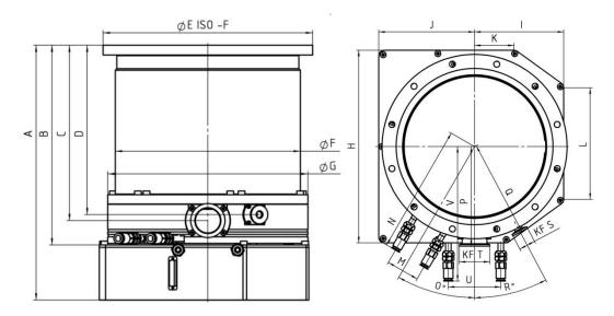
Figure 4.1 Dimensions for CXF-200/1401, CXF-200/1402, CXF-250/2301, CXF-250/2302, CXF-320/3001 and CXF-320/3002
