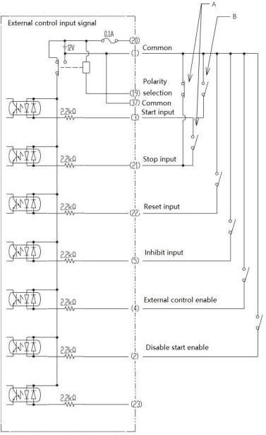
A, B indicate the two methods of table 7.2 Figure 7.4 External control input signal pins (contact input)
