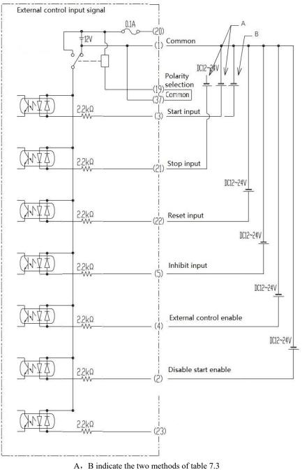
A, B indicate the two methods of table 7.3 Figure 7.5 External control input signal pins (voltage input)
