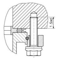
Figure 6.8 Connection of ISO K flange and blind threaded hole
