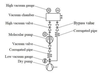
Figure 1.1 Turbomolecular pump applications (vacuum system principle diagram)
