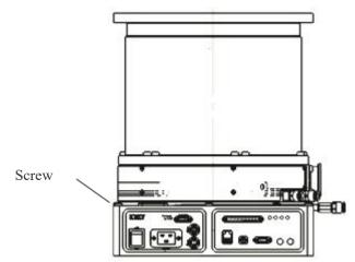
Figure 6.11 Schematic diagram of connecting the integrated controller and turbomolecular pump
