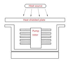
Figure 7.10 Installation diagram of heat shield plate in thermal radiation environment
