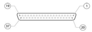
Figure 7.3 I/O external control connector (DB37 pin)
