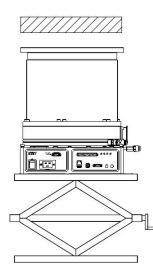
Figure 6.2 Diagram of turbomolecular pump up and down during vertical installation
