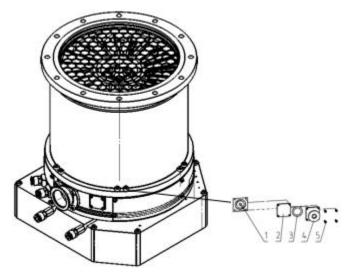
Figure 6.12 Protective gases connections
