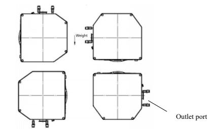
Figure 6.4 Diagram of installation angle of outlet port of integrated magnetically-levitated turbomolecular pump
