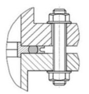
Prior to the flange installation, prepare installation tool, center support, rubber ring, hexagonal bolt and nut, etc. Check the flange sealing surface to ensure that there is no damage;
